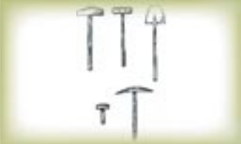
Variety of hammers to break up or shape stones. Spade to remove excess soil from foundation level. Pick or mattock for preparing and digging foundations. 2
