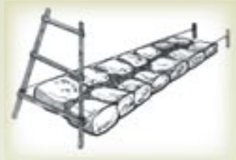
Foundation stones in position. Note the exact alignment of the guide strings.
