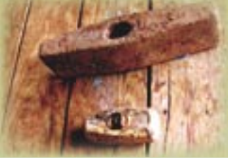
Variety of hammers to break up or shape stones. Spade to remove excess soil from foundation level. Pick or mattock for preparing and digging foundations. 2
