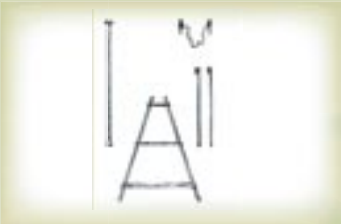
Crow bar used as lever to assist in moving large stones. Walling frame, 'A' frame made from straight-sided timber following the profile or cross section of the wall to be built. Profile bars to maintain correct dimensions. String lines to keep sides straight. 2
